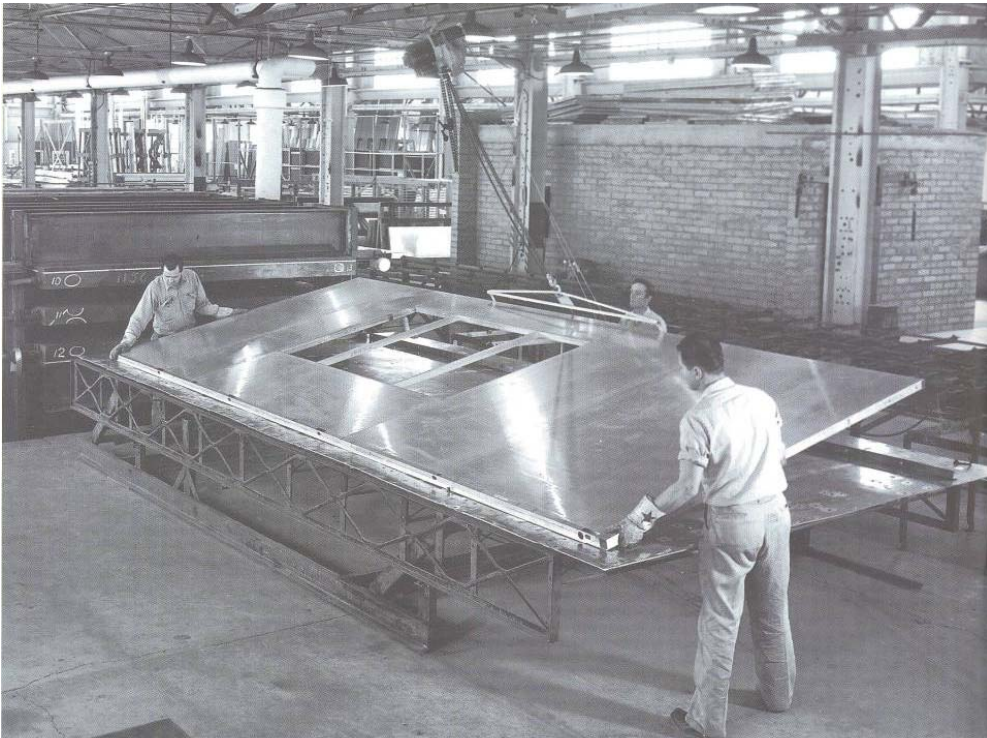
Exterior wall assemblies being set in place during manufacture
